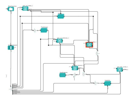
Figure 1: Example of a Reflex workflow, here for UVES echelle mode. The workflow proceeds from left to right. Data are first organized, and then dispatched to the various processing steps. The one that is currently active is highlighted.
